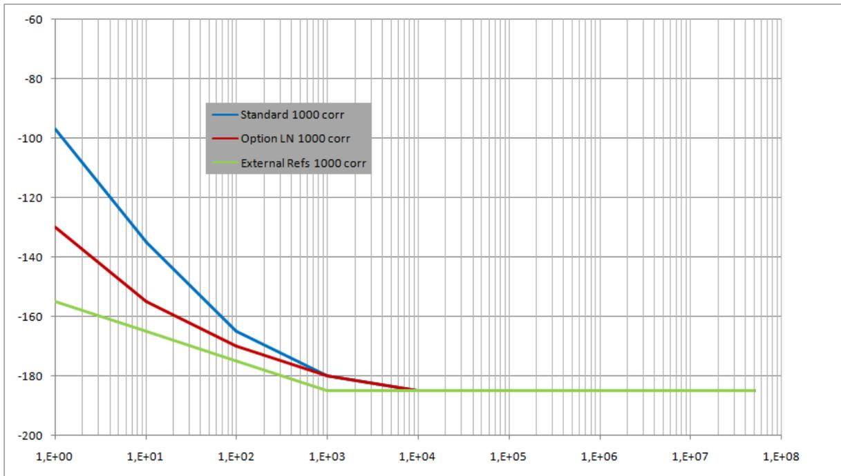
Fig. 2: Phase noise sensitivity of APPH system with different measurement options (1000 correlation, 10 MHz, 5 hours measurement time)
