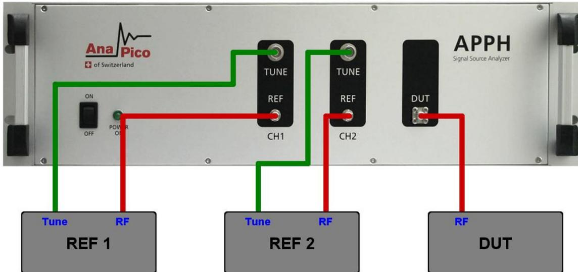
Fig.4: Connectivity block diagram as provided by the APPH GUI software.
