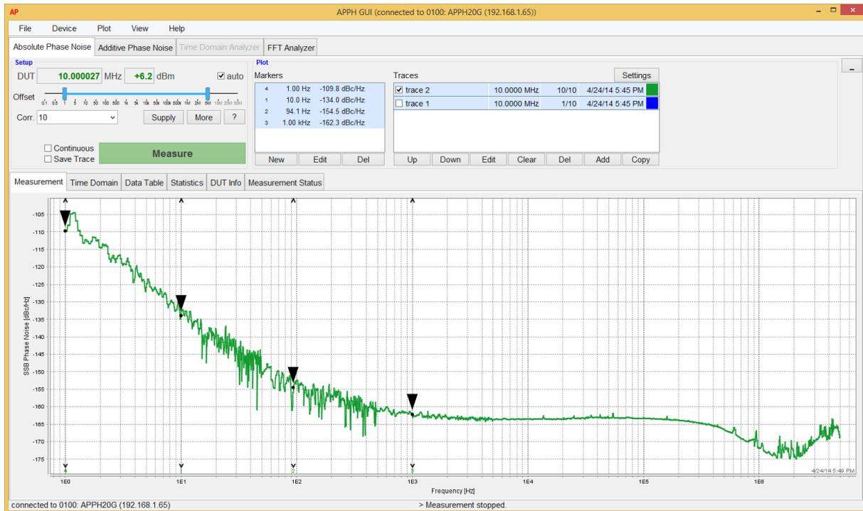
Fig 9: Final measurement after just 10 correlation (160 seconds measurement time).
