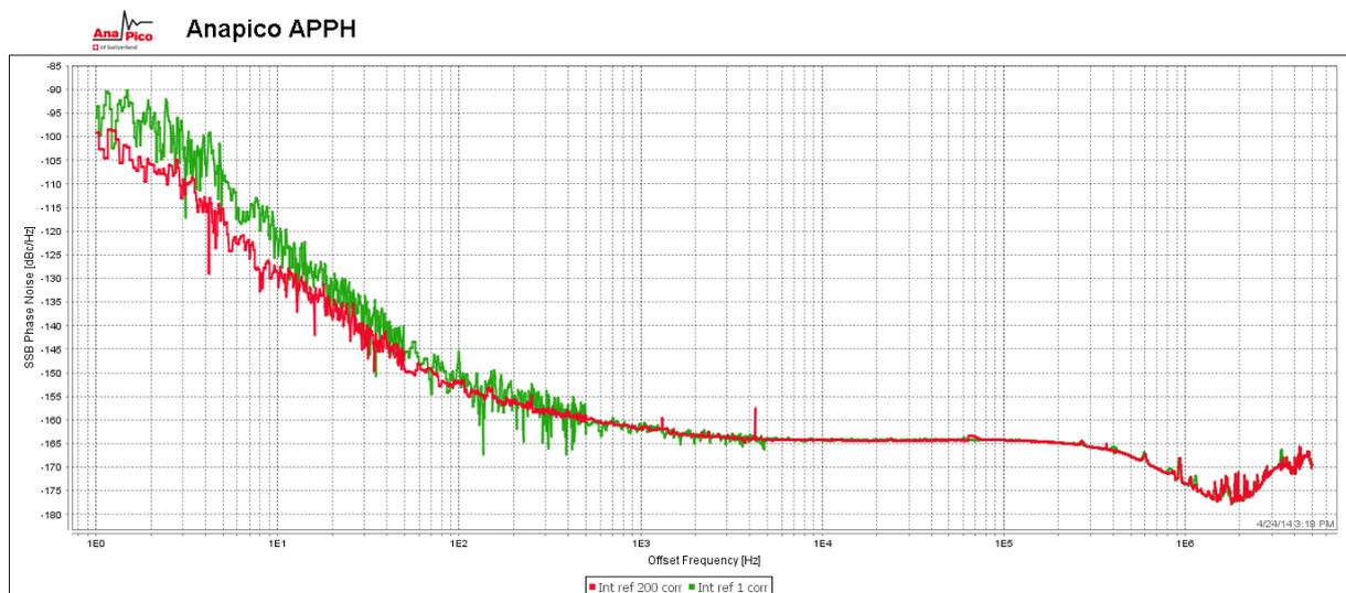
Fig. 3: Phase noise measurement of low-noise 10 MHz OCXO after 1 correlation (green trace) using standard internal references and after 200 correlations (red trace, 90 minutes measurement time).
