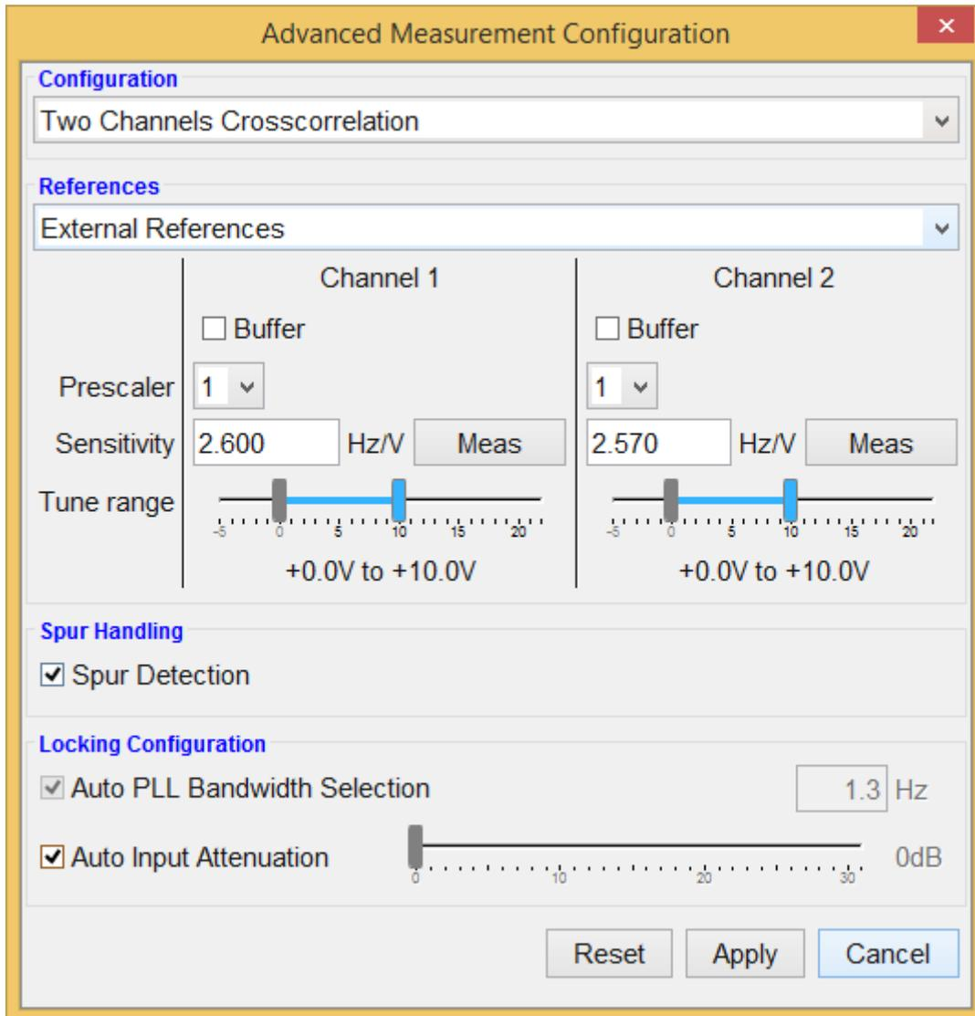
Fig. 7: APPH GUI setup to enable and calibrate external references.
