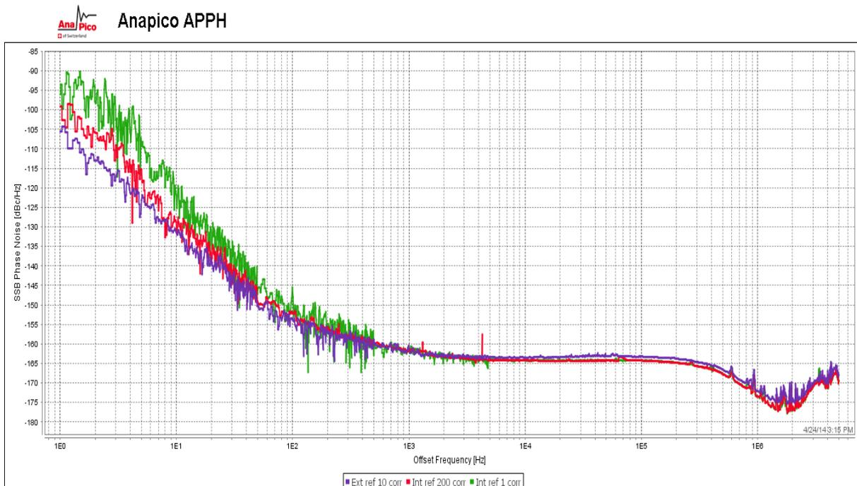
Fig. 10: Phase noise measurement of low-noise 10 MHz with internal references (green and red trace) and external references (purple trace, 10 correlations, 160 seconds measurement time).
