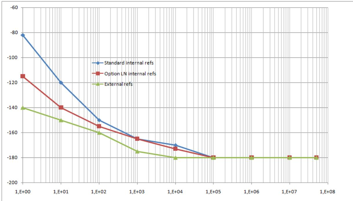
Fig. 1: Phase noise sensitivity of APPH system with different measurement options (1 correlation, 10 MHz, 16 seconds measurement time)
