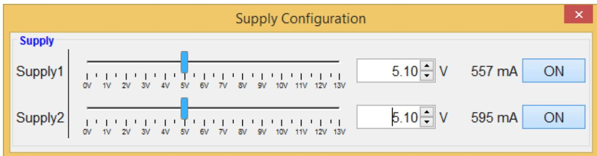
Fig 6: Supply configuration menu. Both supplies are set to 5.1V and during OCXO startup, draw about 550 mA per channel.
